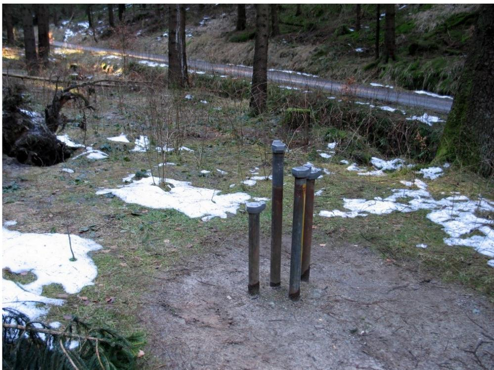
**Figure 21.** Groundwater monitoring pipes in the valley of Nasser Grund.
