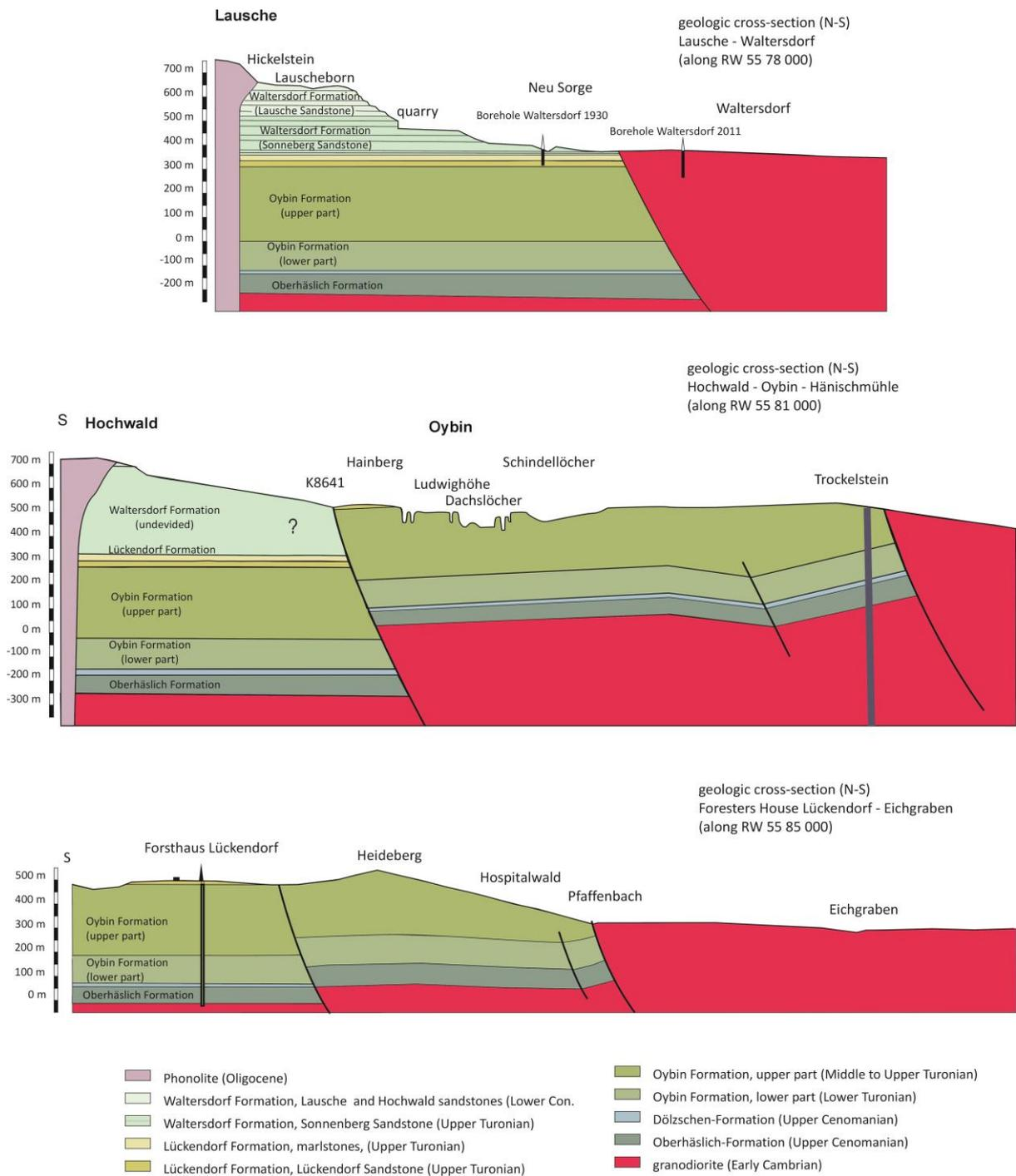
Fig. 7: NS-directed cross-sections across the Lausitz Thrust and the Zittau Mountains show the thick stratigraphic succession of the Cretaceous. Thickness at the Hochwald and the Lausche Hill might exceed 1000 m.
