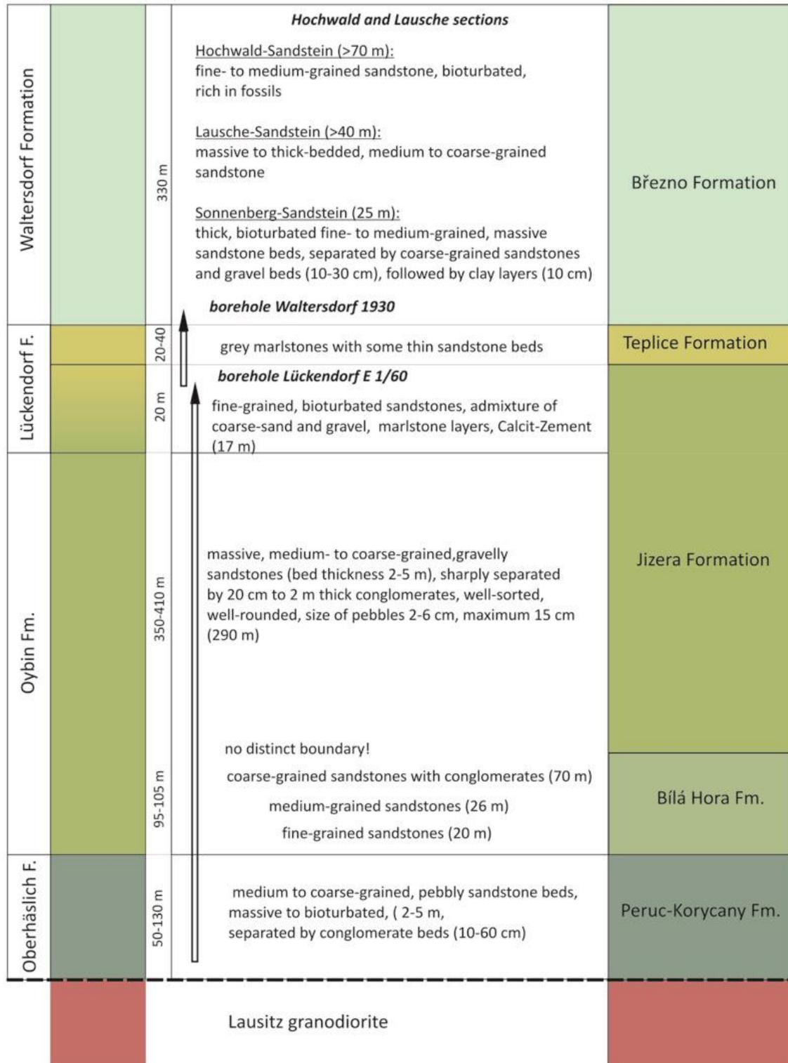
Fig. 6: Combined simplified section of the Cretaceous in the Zittau Mountains. The compilation of several sections allows the correlation with the standard section of the better known Czech side of the Lausche (Dolní Podluží).
