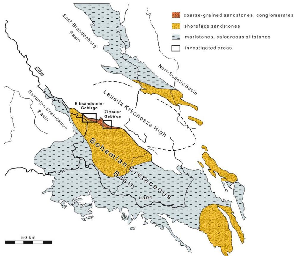
Fig. 1: Overview map of Lausitz-Krkonosze High and the surrounding basins during Turonian. Distribution of sandstones reflects clearly uplift of an isolated source area which was later thrust onto the basin margins. All known deposits are of marine origin; thickness is highest close to the source area, pointing to the formation of marginal troughs. Both the Elbsandsteingebirge and the Zittau Mountains represent depositional systems close to the basin margin. (Figure redrawn from Voigt 2009).
