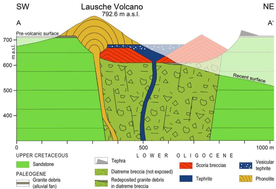
Fig. 11: Reconstructed geological cross-section of the Oligocene Lausche Volcano. A relic of the pre-volcanic surface is marked by granite debris which is preserved by the covering phonolite dome. Weak colouring illustrates erosion since the time of volcanism. See Fig. 10 for position of cross-section A – A'. Figure from WENGER ET AL. (2017).
