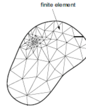
finite element approach (unstructured mesh)
